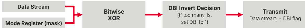
Figure 5. Enhanced Write DBI. Host computes optimal XOR masks, store on mode registers, and inverts/encodes write data to reduce switching/termination power.
